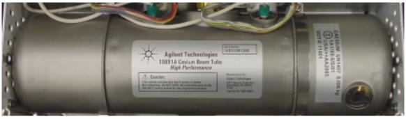
When shipping a 5071A or a replacement CBT in accordance with IATA international DG rules, check the instrument for the above marking. If the marking is present (visible through the cover perforation), follow the IATA international shipping instruction given elsewhere in this website. If the marking is missing, order Label P/N 05071-80030 from Agilent or download from this website. Affix it to the CBT as shown. Follow the shipping instruction referenced above.
